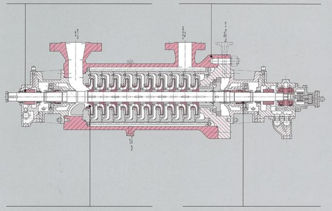
Impellers: The impellers are of the closed type accurately, finished and carefully balanced both statically and dynamicaly. Axial thrust caused by impellers, is balanced by hydraulic balancing devices. Balance drum can be provided instead of balance disk on request. Double suction impeller for first stage is available to reduce NPSH requirements. This seature is available on pump model DCD.
