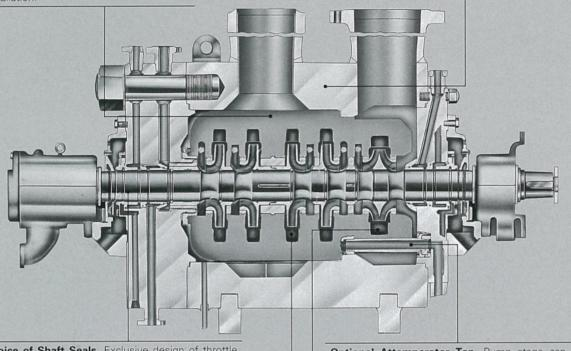
Choice of Shaft Seals. Exclusive design of throttle bushings with cold-condensate injection ensure reliable service, minimum maintenance and remarkably low wear. Also available-conventional packing for lower service requirement...and mechanical seals developed especially for boiler feed service.
